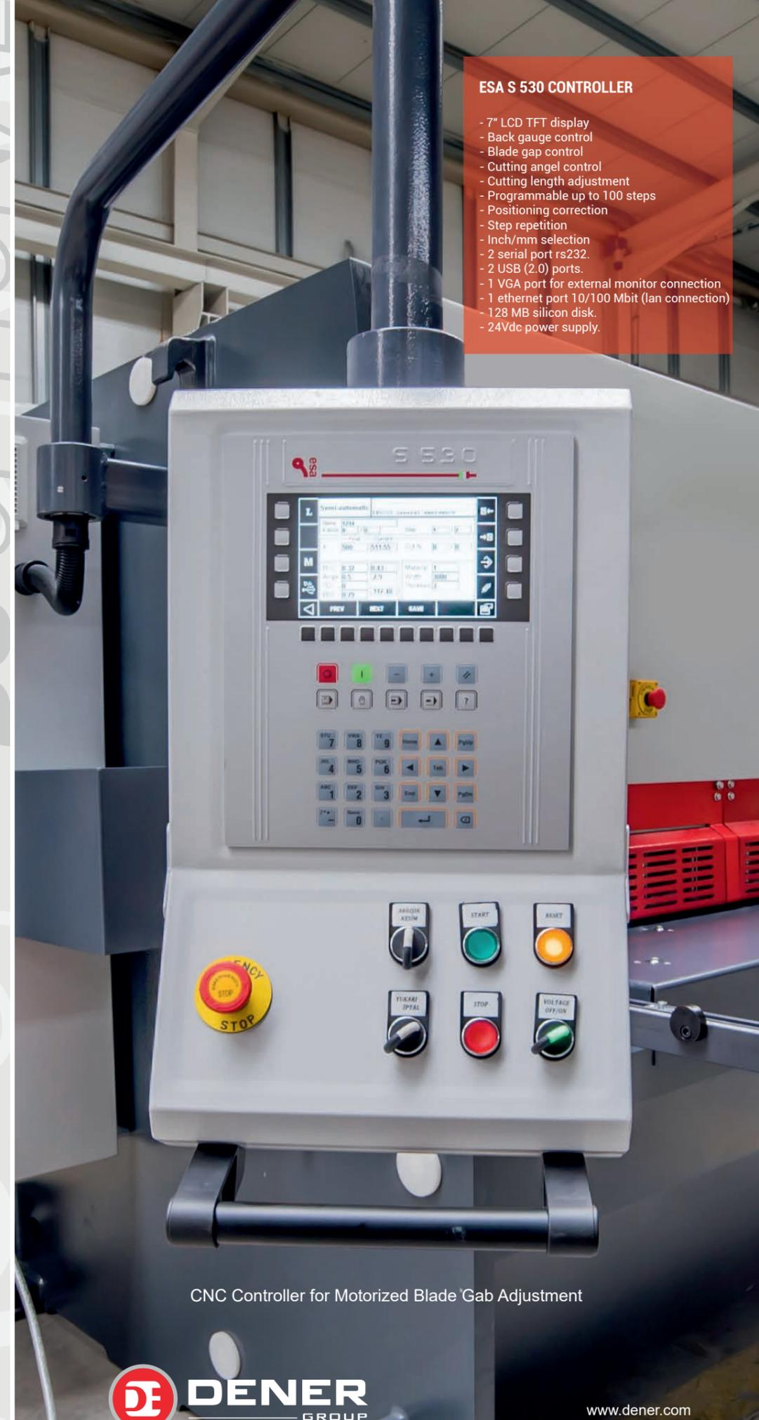
CNC Controller for Motorized Blade Gap Adjustment
