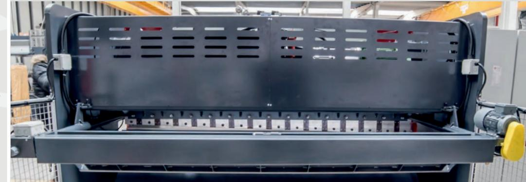
Motorized Back Gauge has  $\pm 0,1$ mm Accuracy
